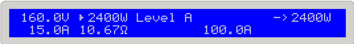
Figure 9. Normal load operation in CP regulation mode
