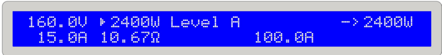
Figure 9. Normal load operation in CP regulation mode
