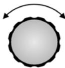
This rotary encoder has no end stop. With every position **Setting (6)** changes the set value resp. the parameter (in the setup menu) which was chosen before by **Selection (5)**.
