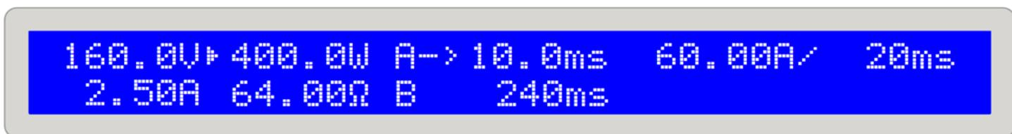
Figure 10. Level A/B operation with pulse width adjustment
