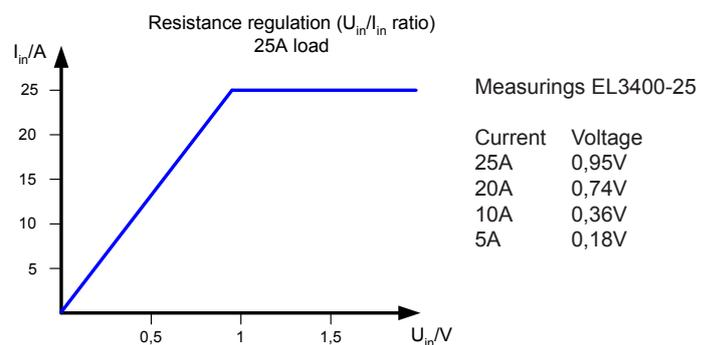
Note: the measured values are taken from final stage transistors of the running production. In case your device has diverging values, it's very probably an older model with different transistors.
