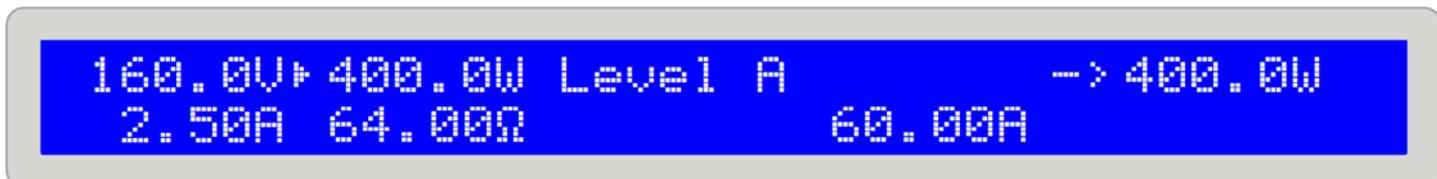
Figure 9. Normal load operation in CP regulation mode
